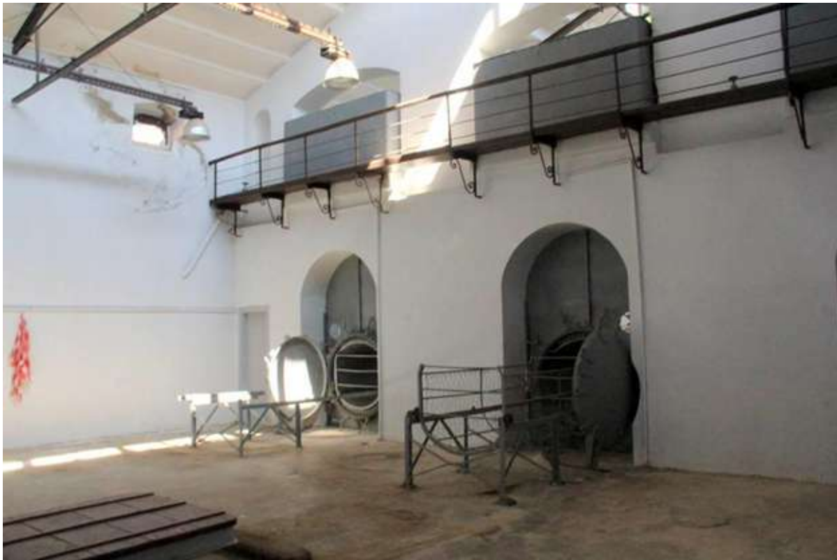
Geneste & Herscher disinfectors (left) disinfection showers (right) preserved in the large station on Urla Karantina Island
